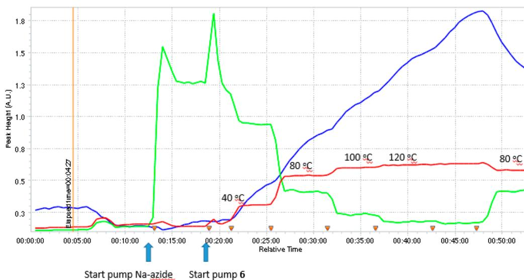
**Figure 4.** Real time FT-IR optimization of the azidoacetate generation. Green line =  $\text{Na-azide}$  ( $2050\text{ cm}^{-1}$ ), Red line =  $\text{azidoacetate 7}$  ( $2112\text{ cm}^{-1}$ ), blue line = temperature.
