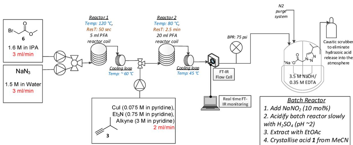
Figure 6. Continuous manufacturing process to obtain carboxylic acid 1.
