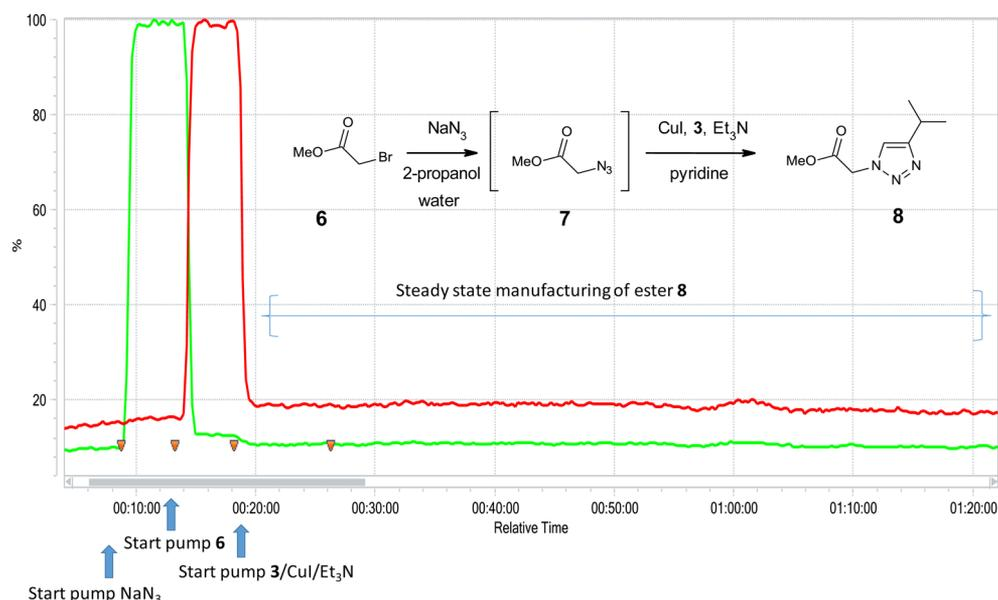
**Figure 7.** FT-IR monitoring of the consumption of Na-azide and azidoacetate 7 in the manufacturing of acid 1. Green line = Na-azide ( $2050\text{ cm}^{-1}$ ), red line = azidoacetate 7 ( $2112\text{ cm}^{-1}$ ).
