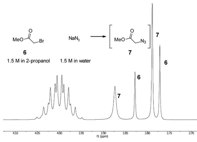
this solvent composition was also well suited for the azidoacetate generation, and at reflux, full and clean conversion was obtained within 1 h. The solvent composition was also appropriate for long time storage of **7**, as we did not see any decomposition or precipitation after aging for a few days at 20 °C.
