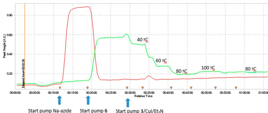
Figure 5. Real time FT-IR optimization of the cycloaddition. Red line = Na-azide ( $2050\text{ cm}^{-1}$ ), Green line = azidoacetate 7 ( $2112\text{ cm}^{-1}$ ).
