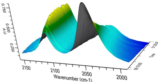
**Figure 2.** FT-IR monitoring of azidoacetate generation **7** ( $2112\text{ cm}^{-1}$ ) from **6** and  $\text{NaN}_3$  ( $2050\text{ cm}^{-1}$ ).
