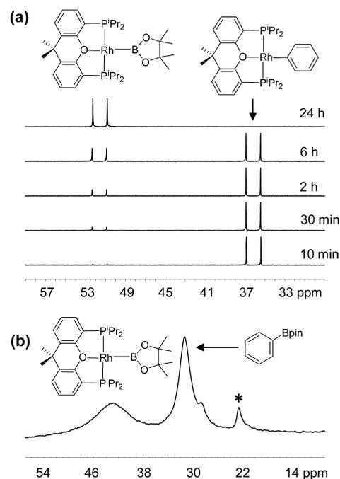
**Figure 5.** (a) Stacked  $^{31}\text{P}\{^1\text{H}\}$  NMR spectra showing the transformation of  $\text{RhPh}\{\text{xant}(\text{P}^i\text{Pr}_2)_2\}$  (**2**) into  $\text{Rh}(\text{Bpin})\{\text{xant}(\text{P}^i\text{Pr}_2)_2\}$  (**9**) by reaction with  $\text{B}_2\text{pin}_2$  (toluene, 60 °C). (b)  $^{11}\text{B}\{^1\text{H}\}$  NMR spectrum of the reaction after 24 h at 60 °C. \*  $\text{B}_2\text{pin}_3$  (decomposition product).
