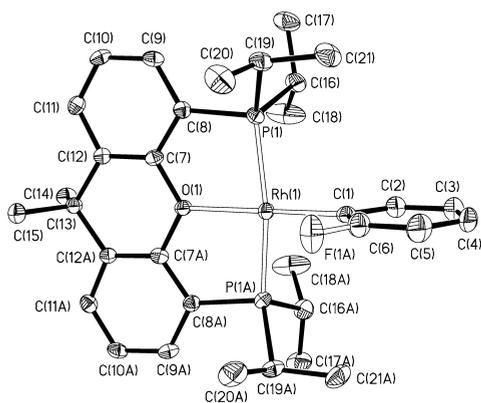
**Figure 2.** ORTEP diagram of complex **5** (50% probability ellipsoids). Hydrogen atoms are omitted for clarity. Selected bond lengths (Å) and angles (deg): Rh(1)–P(1) = 2.2520(8), Rh(1)–O(1) = 2.193(3), Rh(1)–C(1) = 1.994(4); P(1)–Rh(1)–P(1A) = 161.13(4), P(1)–Rh(1)–O(1) = 82.73(2), P(1A)–Rh(1)–O(1) = 82.73(2), O(1)–Rh(1)–C(1) = 179.90(14).
