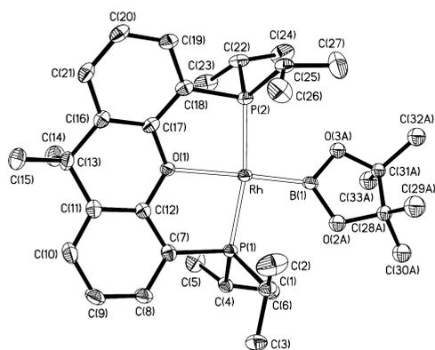
**Figure 4.** ORTEP diagram of complex **9** (50% probability ellipsoids). Hydrogen atoms are omitted for clarity. Selected bond lengths (Å) and angles (deg): Rh–P(1) = 2.2255(9), Rh–P(2) = 2.2432(9), Rh(1)–O(1) = 2.268(2), Rh–B(1) = 1.981(4); P(1)–Rh(1)–P(2) = 161.98(3), P(1)–Rh–O(1) = 83.07(6), P(2)–Rh–O(1) = 82.98(6), O(1)–Rh(1)–C(1) = 177.22(14).
