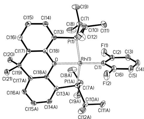
**Figure 3.** ORTEP diagram of complex **6** (50% probability ellipsoids). Hydrogen atoms are omitted for clarity. Selected bond lengths (Å) and angles (deg): Rh(1)–P(1) = 2.2521(3), Rh(1)–O = 2.1850(13), Rh(1)–C(1) = 1.9898(19); P(1)–Rh(1)–P(1A) = 161.611(18), P(1)–Rh(1)–O(1) = 82.782(10), P(1A)–Rh(1)–O(1) = 82.781(10), O(1)–Rh(1)–C(1) = 179.45(6).
