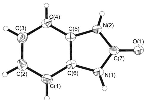
**Figure 1** Thermal ellipsoid (30%) plot of complex **3aa**. Selected bond lengths (Å) and angles (°): N(1)–C(7) 1.356(3), N(1)–C(6) 1.387(2), N(2)–C(7) 1.361(2), N(2)–C(5) 1.386(3), O(1)–C(7) 1.240(2), C(7)–N(1)–C(6) 110.2(2), C(7)–N(2)–C(5) 110.0(2), O(1)–C(7)–N(1) 126.8(2), O(1)–C(7)–N(2) 126.5(2), N(1)–C(7)–N(2) 106.7(2).
