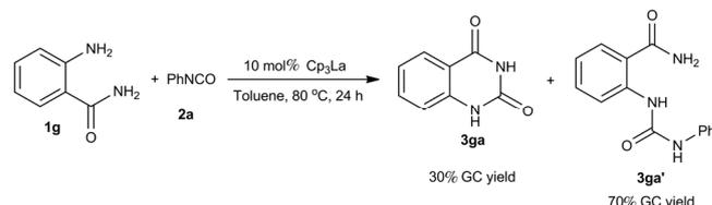
**Scheme 1**  $\text{Cp}_3\text{La}$  catalyzed cyclocarbonylation.
