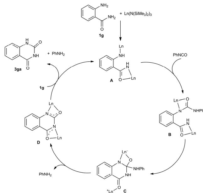
**Scheme 3** Possible mechanism of cyclization between diamines and isocyanates.
