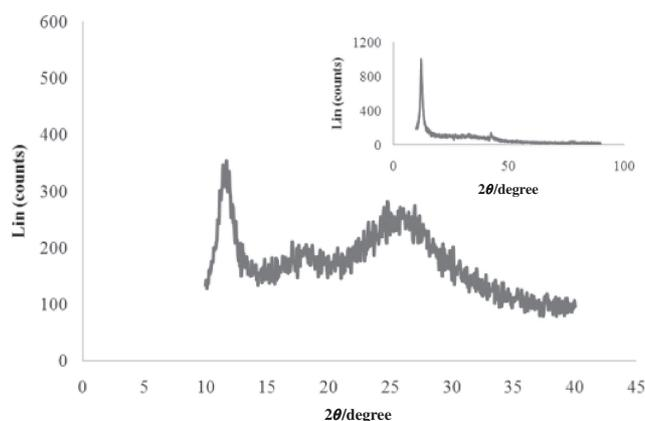
**Figure 2.** XRD patterns of separated GO after oxidation of benzyl alcohol and GO (inset).
