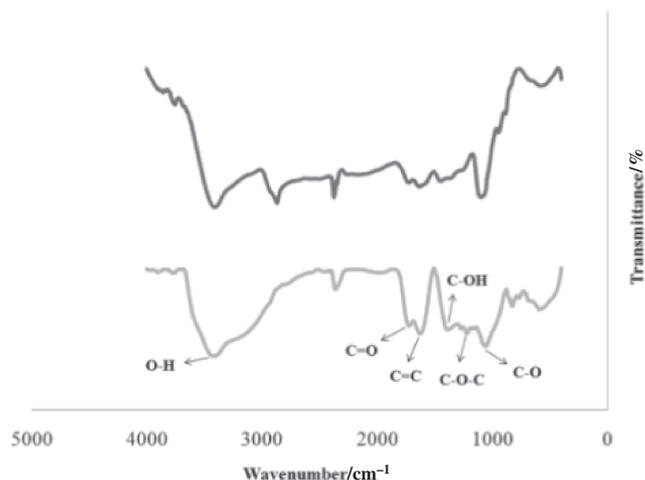
**Figure 1.** IR spectrum of separated GO (up) after oxidation of benzyl alcohol and fresh GO (down).
