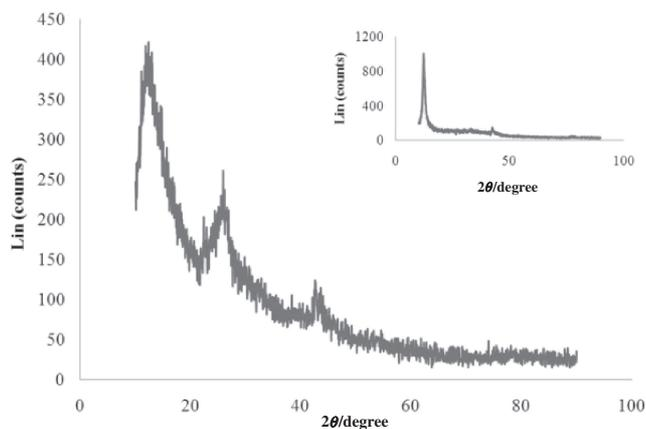
**Figure 4.** XRD patterns of GO and GO after 1 run of reaction (inset).
