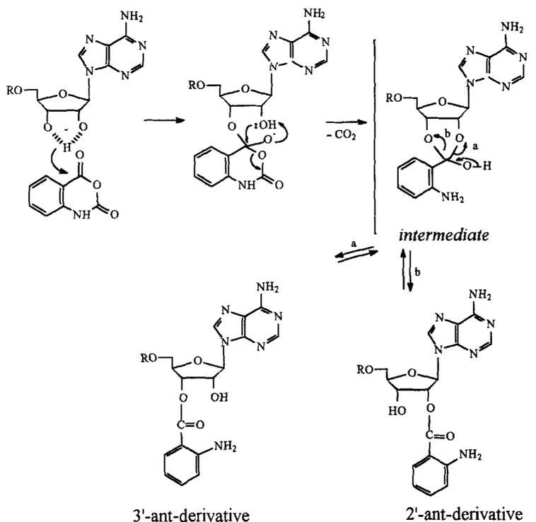
FIG. 8. Proposed mechanism of the reaction between the 2'(3')-cis-diol function of the ribose moiety of nucleotides or nucleosides and isatoic anhydride in basic aqueous medium.
