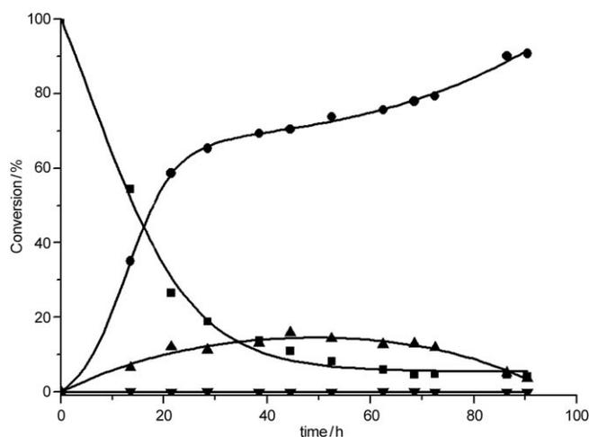
**Figure 2.** Production distribution over time (for reaction conditions see Table 2). ■: cyclohexanol, ●: cyclohexylamine, ▲: dicyclohexylamine, ▼: cyclohexanone.
