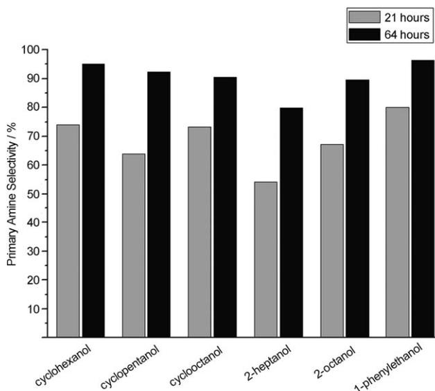
**Figure 3.** Primary amine selectivity for different substrates after 21 and 64 h. For cyclohexanol the selectivities are given after 21 and 92 h. Reaction conditions: substrate (10 mmol),  $[\text{Ru}_3(\text{CO})_{12}]$  (0.1 mmol), ligand **6** (0.6 mmol), cyclohexane (6 mL),  $\text{NH}_3$  (l) (6 mL),  $140^\circ\text{C}$ ,  $([\text{Ru}_3(\text{CO})_{12}]/\mathbf{6}/\text{substrate}) = 1:6:100$ .
