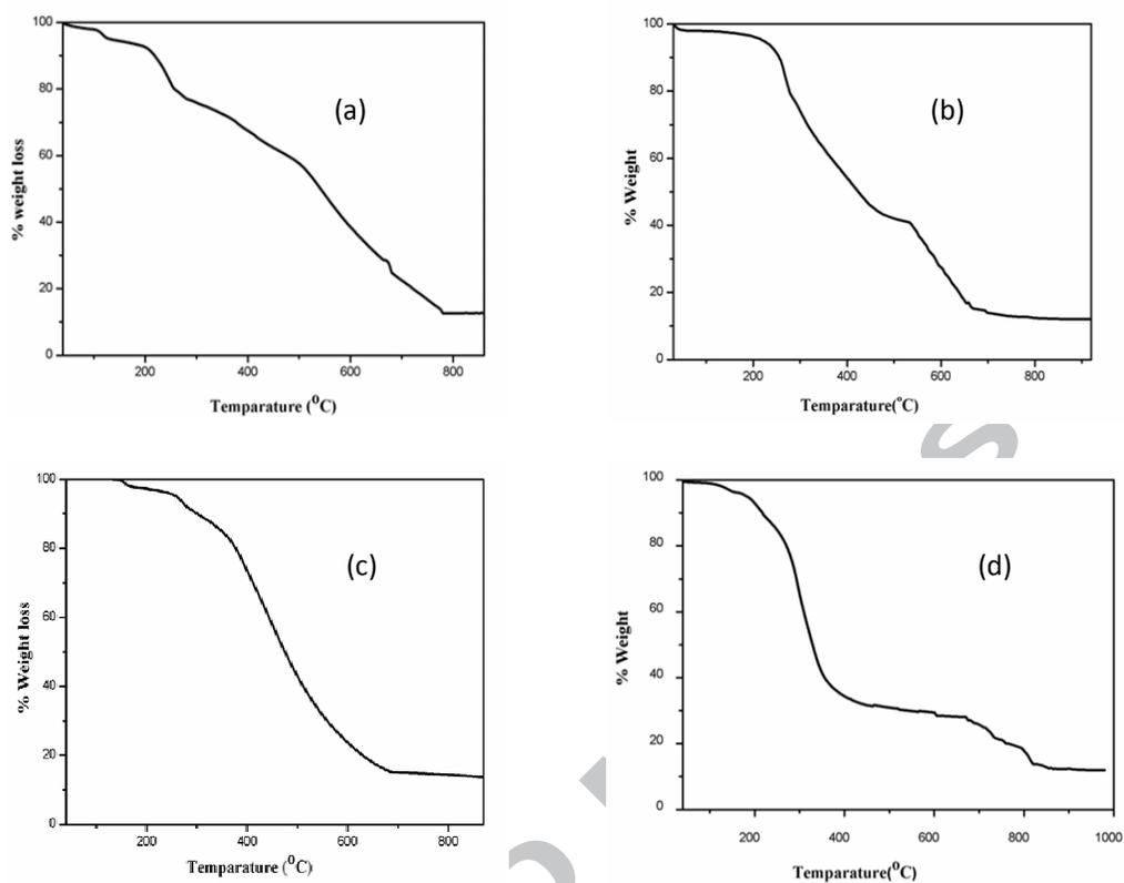
Figure 4. TG graphs of (a)  $[\text{Cu}(\text{L}_1)_2] \cdot 2\text{H}_2\text{O}$ , (b)  $[\text{Cu}(\text{L}_2)_2] \cdot \text{H}_2\text{O}$ , (c)  $[\text{Cu}(\text{L}_3)_2]$ , (d)  $[\text{Cu}(\text{L}_4)_2]$
