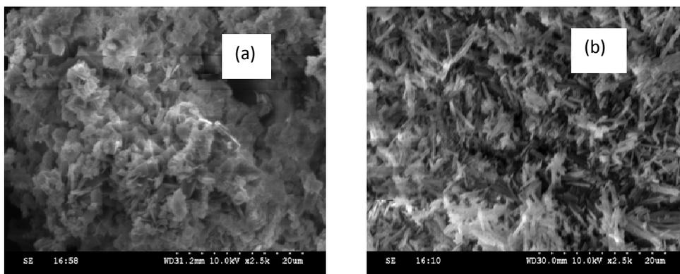
Figure 8. SEM micrographs of (a)  $[\text{Cu}(\text{L}_1)_2] \cdot 2\text{H}_2\text{O}$  (b)  $[\text{Cu}(\text{L}_3)_2]$
