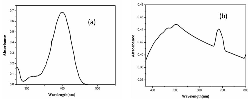
Figure 2. Electronic spectra of (a) HL<sub>1</sub> (b) [Cu(L<sub>1</sub>)<sub>2</sub>].2H<sub>2</sub>O
