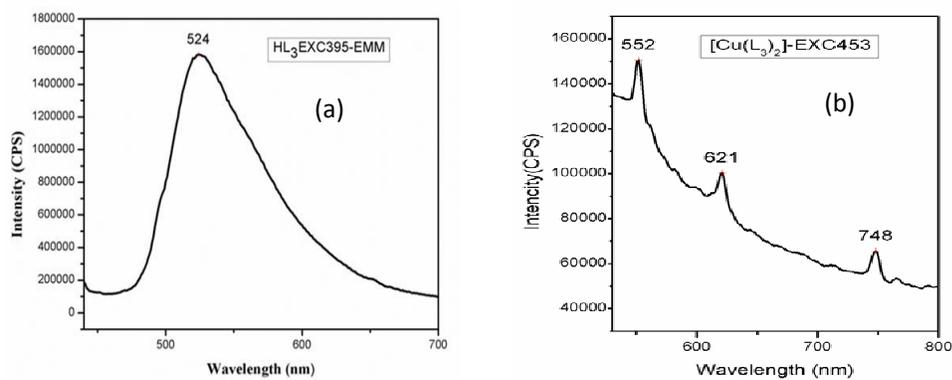
Figure 6. Emission spectra of (a) HL<sub>3</sub> (b) [Cu(L<sub>3</sub>)<sub>2</sub>]
