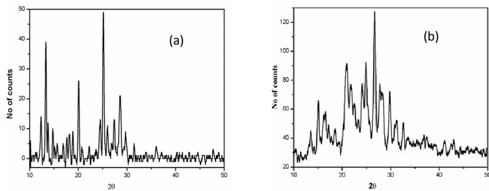
Figure 7. PXRD patterns of (a) HL<sub>3</sub> (b) [Cu(L<sub>3</sub>)<sub>2</sub>]
