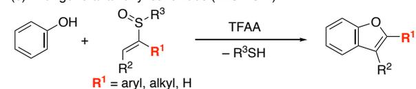
**Scheme 1.** Pummerer annulation for synthesis of benzofurans
