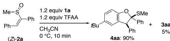
**Scheme 3.** Synthesis of 2-sulfanyl-2,3-dihydrobenzofuran **4aa** in CH<sub>3</sub>CN.
