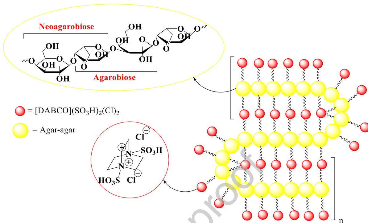
**Figure 1.** Agar/agarose structure and agar-entrapped sulfonated DABCO
