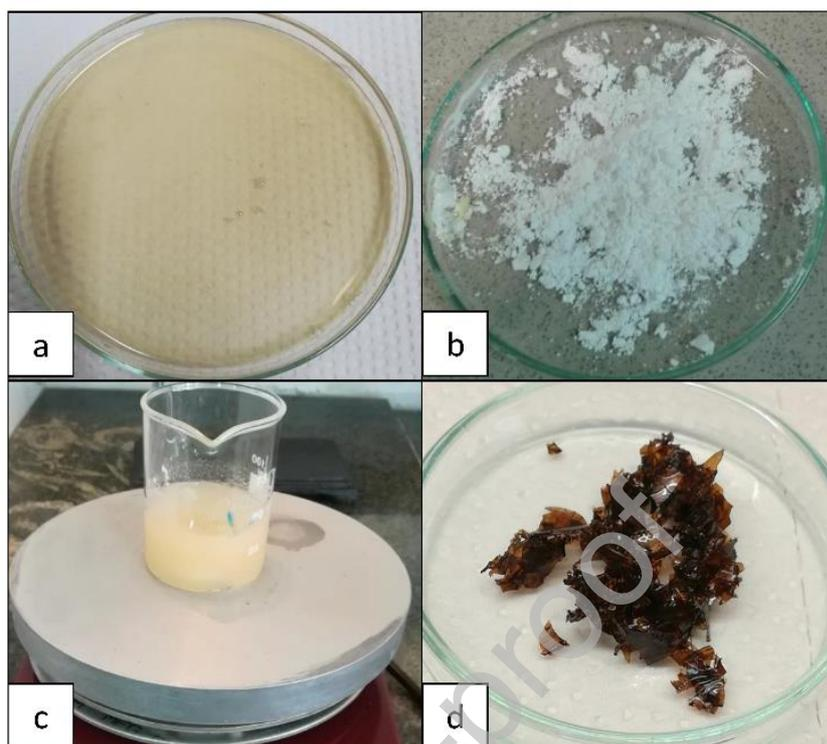
**Figure 3.** Agar in heated water (a),  $[\text{DABCO}](\text{SO}_3\text{H})_2(\text{Cl})_2$  (b), ionic liquid in warm water (c) and agar-entrapped ionic liquid (d).
