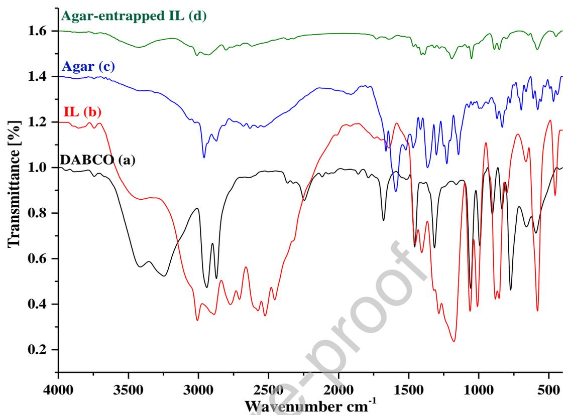
Figure 5. FT-IR spectra of DABCO (a), [DABCO] ( $\text{SO}_3\text{H}$ ) $_2\text{Cl}_2$  (b), agar (c) and agar-entrapped IL (d)
