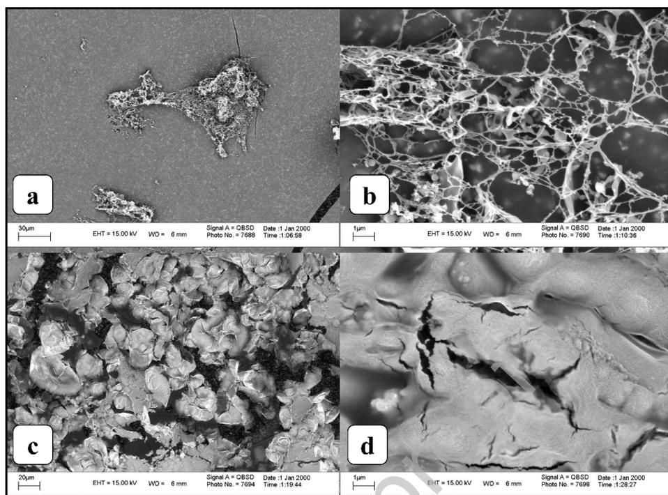
**Figure 6.** SEM of DABCO (a and b) and agar-entrapped IL (c and d)
