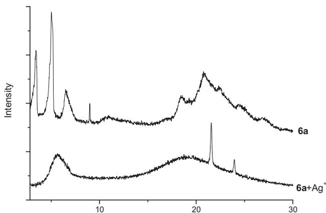
Figure 6. XRD traces of neat triad **6a** and its complex at 70 °C.
