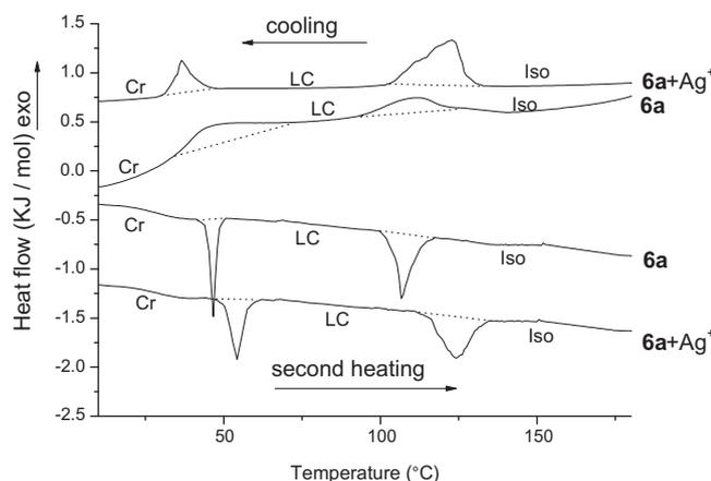
**Figure 2.** The DSC traces of **6a** and complex **6a+Ag<sup>+</sup>** on second heating and cooling (scan rate  $10\text{ }^\circ\text{C min}^{-1}$ ).
