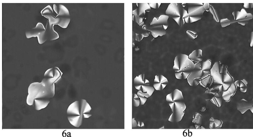
Figure 4. The textures of **6a** and **6b** under POM on cooling at 70 °C ( $\times 400$ ).
