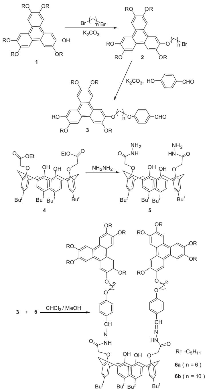
**Scheme 1.** The synthetic route of novel triads of triphenylene-calix[4]arene-triphenylenes **6a** and **6b**.
