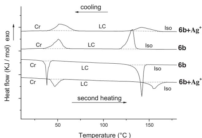
**Figure 3.** The DSC traces of **6b** and complex **6a+Ag<sup>+</sup>** on second heating and cooling (scan rate  $10\text{ }^\circ\text{C min}^{-1}$ ).
