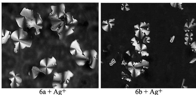
Figure 5. The textures of complexes **6a** and **6b** with  $\text{AgClO}_4$  under POM on cooling at 70 °C ( $\times 400$ ).
