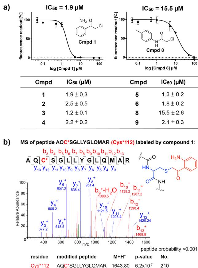
**Figure 3.** Inhibition of PqsD *in situ*. (a) Dose–response curves of compounds **1** and **8** and IC<sub>50</sub> values of all active compounds. (b) Tryptic peptide fragment with compound **1** covalently bound to the active site cysteine of PqsD after *in situ* inhibition.
