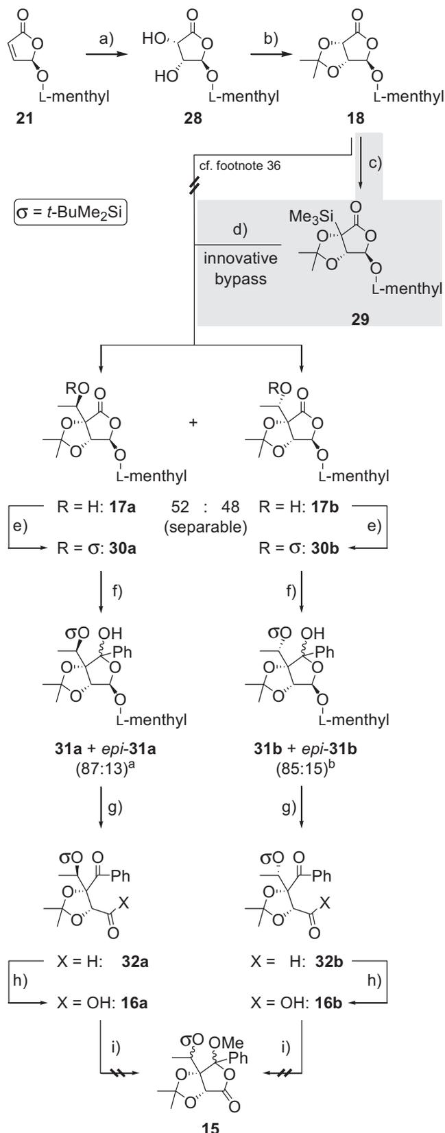
**Scheme 2.** Conversion of the Feringa lactone (**21**) into the furanone **18** and into the  $\gamma$ -keto-carboxylic acid (**16a,b**) equivalents of the furanones **15**, precursors of the
