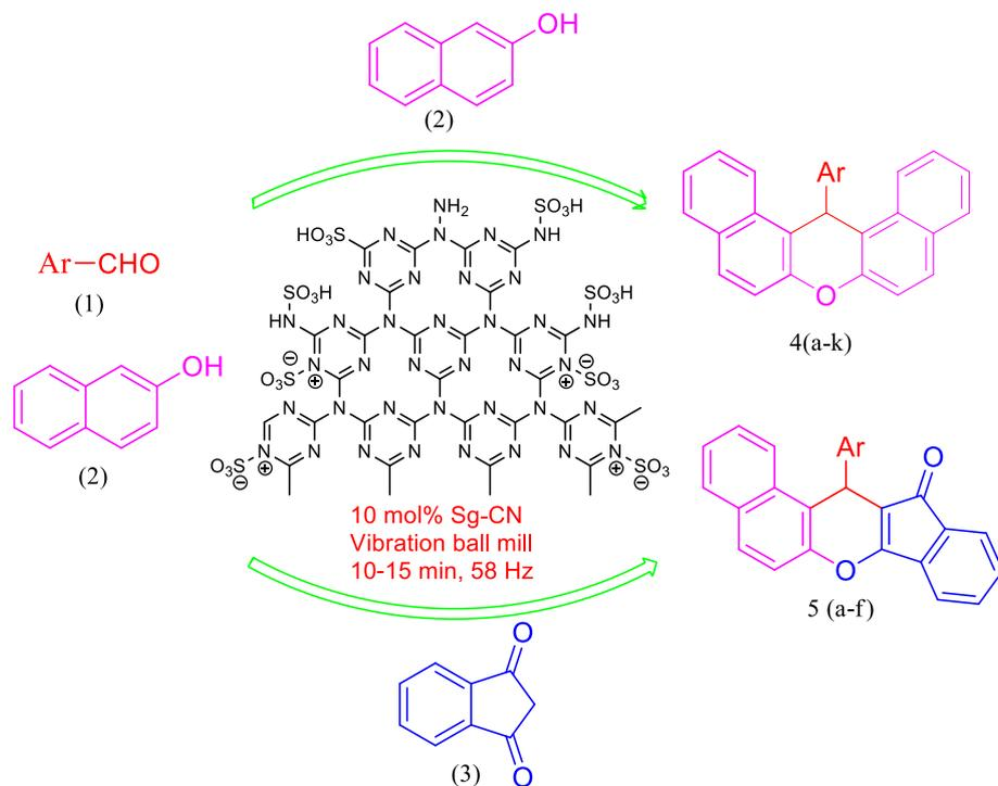
SCHEME 1 One-pot synthesis of xanthene derivatives using Sg-CN in a vibration ball-mill
