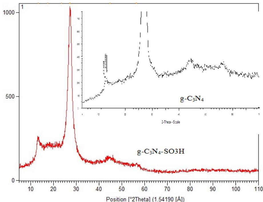
FIGURE 3 XRD patterns for g-C<sub>3</sub>N<sub>4</sub> and g-C<sub>3</sub>N<sub>4</sub>-SO<sub>3</sub>H
