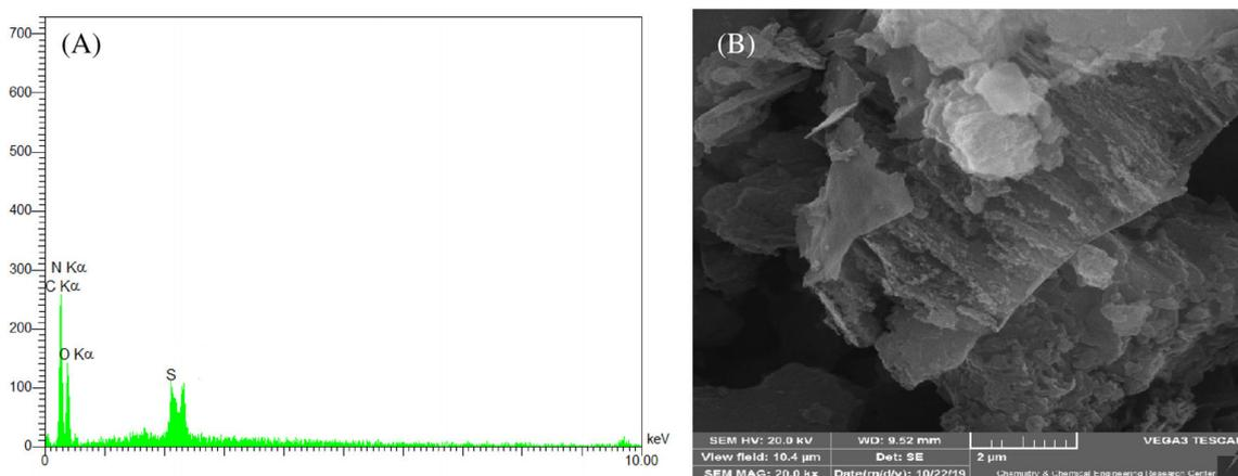
FIGURE 2 (A) EDX mapping of Sg-CN and (B) SEM images Sg-CN
