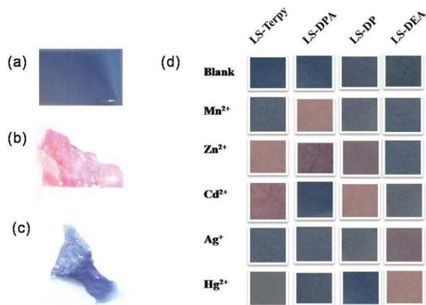
**Fig. 9** (a) Transparent blue colour PVA film with embedded **LS-DPA** receptor (b) PVA film with embedded **LS-DPA** receptor in the presence of zinc ions (c) with cadmium ions in water (d) test papers prepared from different vesicular solutions in presence and absence of metal ions.
