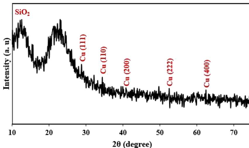
FIGURE 5 X-ray diffraction (XRD) patterns of Cu(II) Schiff-base@silica as a nanocatalyst
