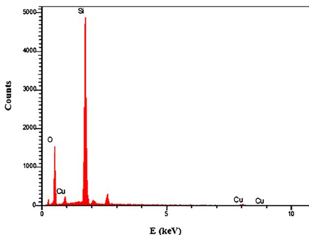
FIGURE 4 Energy-dispersive X-ray spectroscopy (EDX) of Cu(II) Schiff-base@SiO<sub>2</sub>
