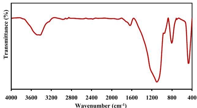
FIGURE 7 Infrared (IR) spectrum for the Cu(II) Schiff-base@SiO<sub>2</sub> after the 10 cycles
