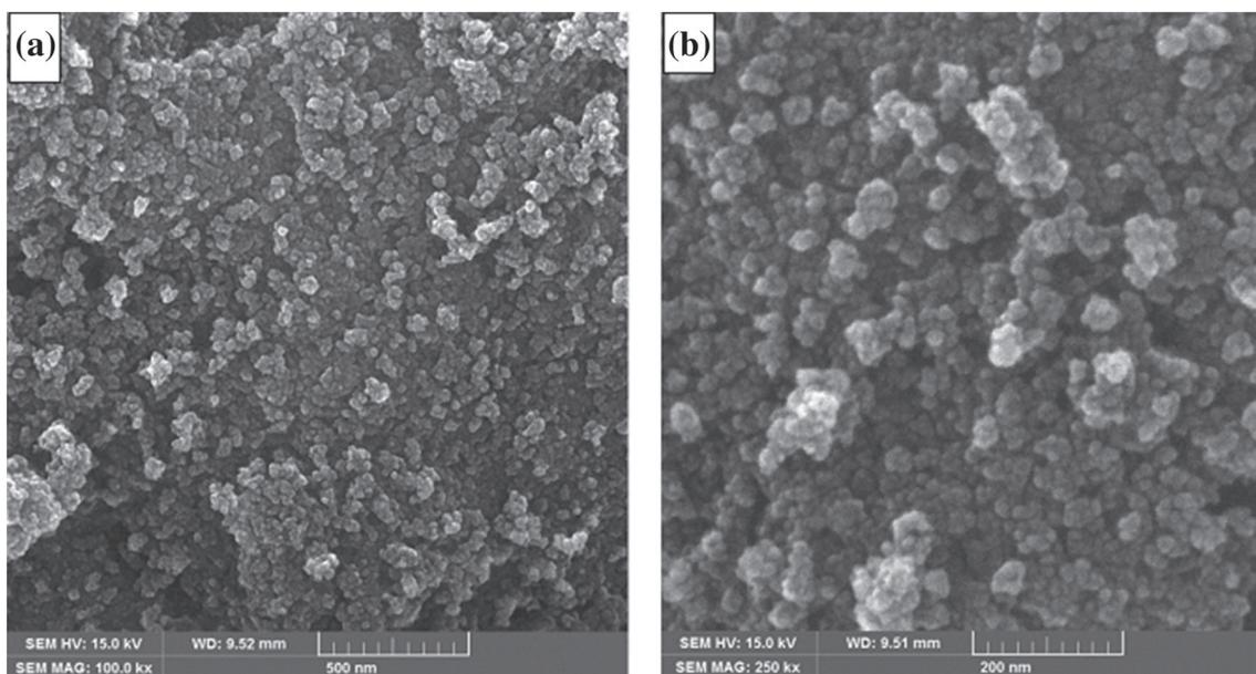
FIGURE 3 Field emission scanning electron microscope (FESEM) images of Cu(II) Schiff-base@SiO<sub>2</sub>
