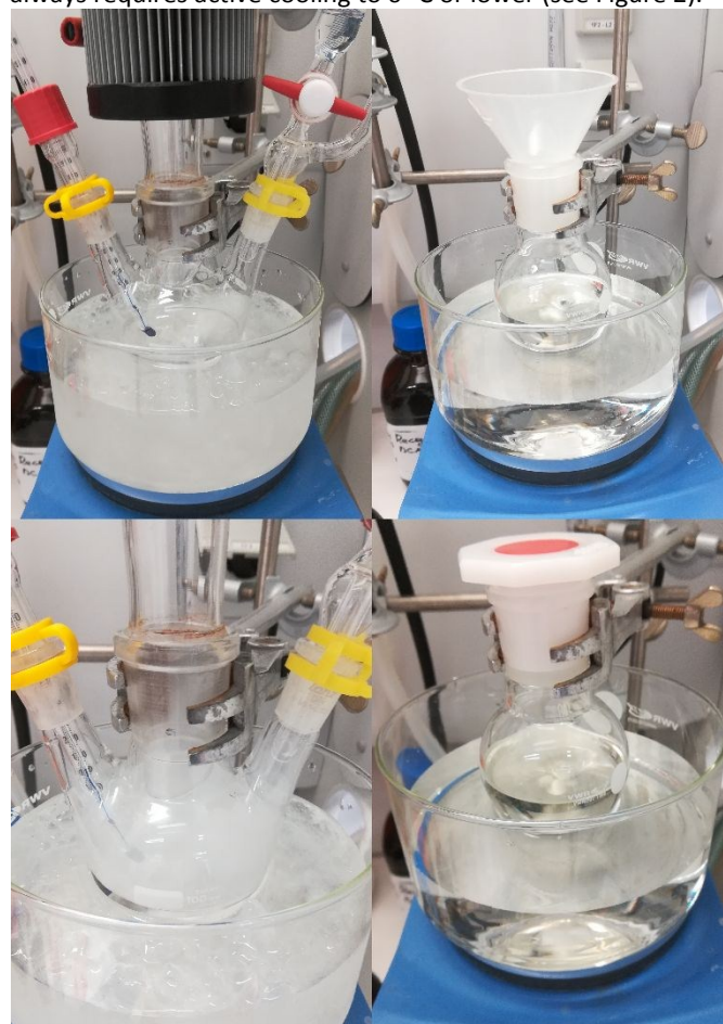
Figure 2: Top left: Dehydration of tert -butyl formamide (11.6 mmol in 35 mL DCM, (0.33 M)), cooling is applied for subsequent addition of \text{POCl}_3 . Bottom left: Reaction after addition of \text{POCl}_3 , internal temperature at 0 °C, still HCl vapors are evolving. Top right: Dehydration of tert -butyl formamide (35 mmol in 35 mL DCM, 1.00 M), a water bath is applied for subsequent addition of p -TsCl. Bottom right: Reaction after addition of p -TsCl. No visible hints of an exothermic reaction are observed. In some dehydrations, the temperature increased slightly.
