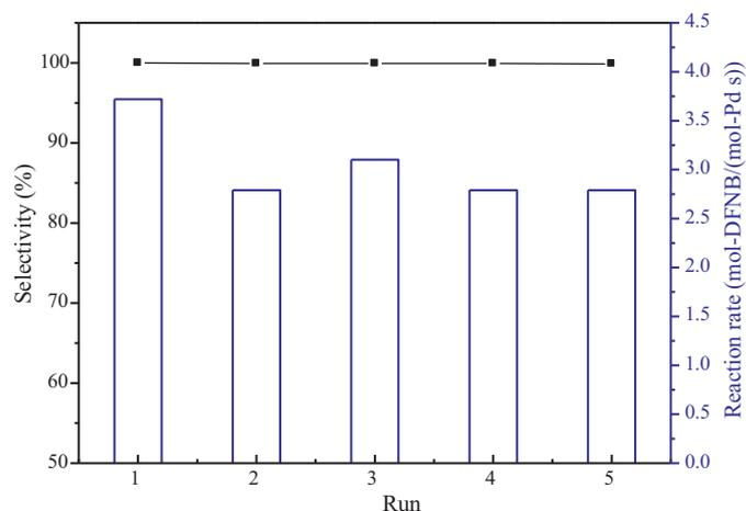
Fig. 5. The recycling results for Pd/SnO<sub>2</sub>/C catalyst in the hydrogenation of DFNB.
