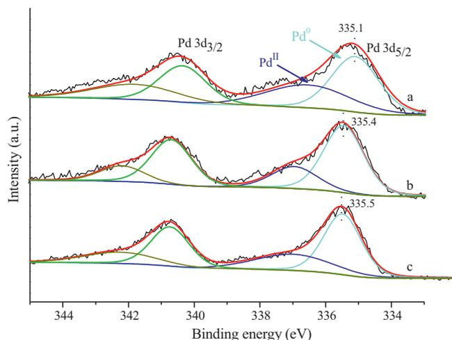
Fig. 4. Pd 3d photoemission core-level spectra for (a) Pd/C, (b) Pd/SnO<sub>2</sub> and (c) Pd/SnO<sub>2</sub>/C.
