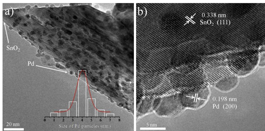
Fig. 1. (a) TEM image of Pd/SnO<sub>2</sub>/C and the crystallite size distribution and (b) HRTEM image of Pd/SnO<sub>2</sub>/C.
