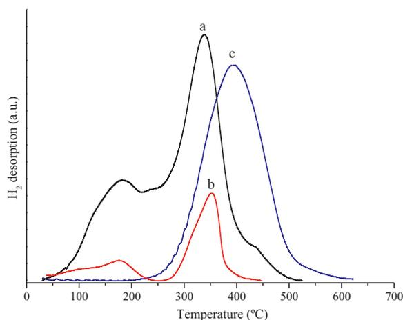
Fig. 3. H<sub>2</sub> TPD profiles of (a) Pd/SnO<sub>2</sub>/C, (b) Pd/SnO<sub>2</sub>, and (c) Pd/C.
