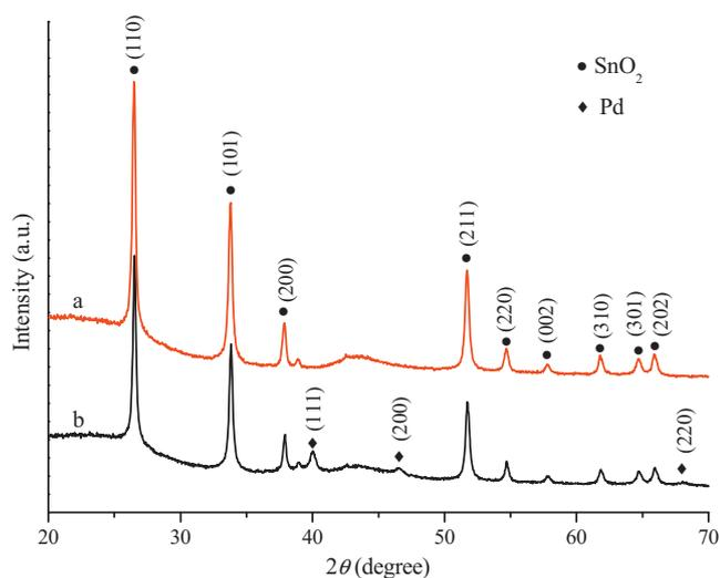
Fig. 2. XRD patterns of (a) SnO<sub>2</sub>/C and (b) Pd/SnO<sub>2</sub>/C.
