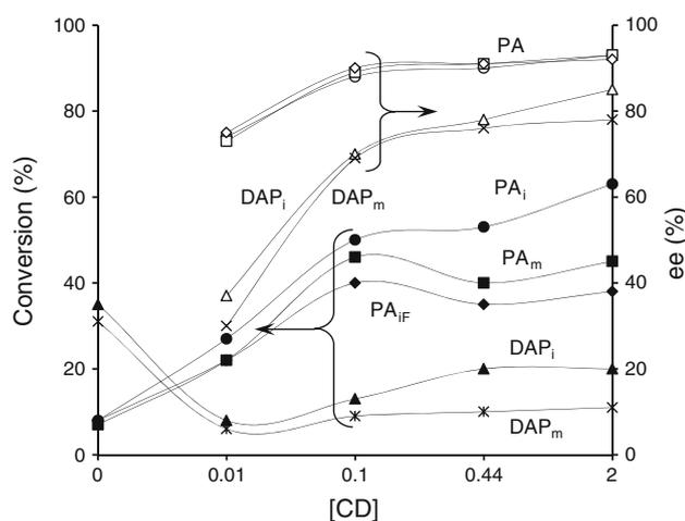
**Fig. 1** Enantioselective hydrogenation of PA, DAP and their binary mixture: effect of the modifier concentration on the conversion (closed symbols) and on ee (open symbols); (subscript *i* individual, *m* mixture, *iF* final individual hydrogenation, see Sect. 2.2)
