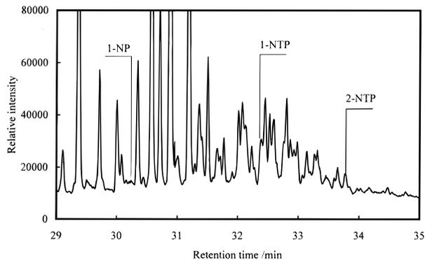
FIGURE 1. Gas chromatogram with NPD of the 12/9 nighttime samples. The identity of the peaks are as follows: 1-NP, 1-nitropyrene; 1-NTP, 1-nitrotriphenylene; and 2-NTP, 2-nitrotriphenylene.
