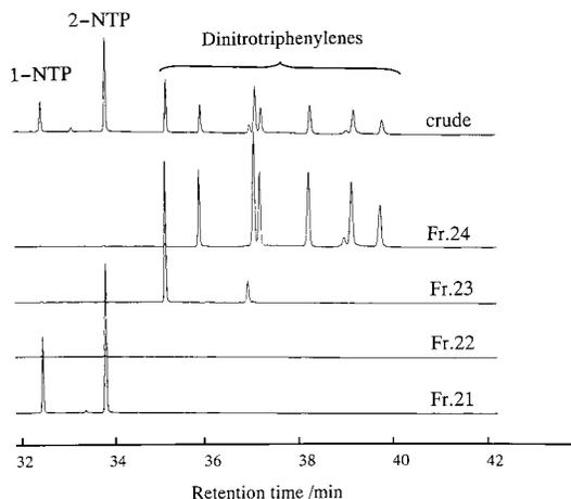
FIGURE 9. Gas chromatograms of the crude sample and HPLC fractions from 21 to 24 in the dark reaction product in the presence of  $O_3$  for 24 h.
