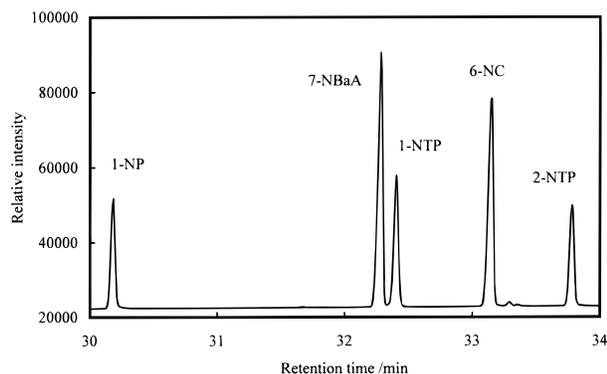
FIGURE 2. Gas chromatogram with NPD showing resolution of 1- and 2-nitrotriphenylenes (1- and 2-NTPs), 7-nitrobenz[a]anthracene (7-NBaA), and 6-nitrochrysene (6-NC). 1-Nitropyrene and the isomers in order of elution are as follows: 1-nitropyrene, 7-nitrobenz[a]anthracene, 1-nitrotriphenylene, 6-nitrochrysene, and 2-nitrotriphenylene.
