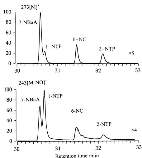
FIGURE 3. Mass chromatograms for molecular ions ( $m/z$  273) and the  $[M - NO]^+$  ( $m/z$  243) fragment ions from the GC/MS-SIM analysis, showing resolution of 1- and 2-nitrotriphenylenes (1- and 2-NTPs), 7-nitrobenz[a]anthracene (7-NBaA), and 6-nitrochrysene (6-NC). The isomers in order of elution are as follows: 7-nitrobenz[a]anthracene, 1-nitrotriphenylene, 6-nitrochrysene, and 2-nitrotriphenylene.
