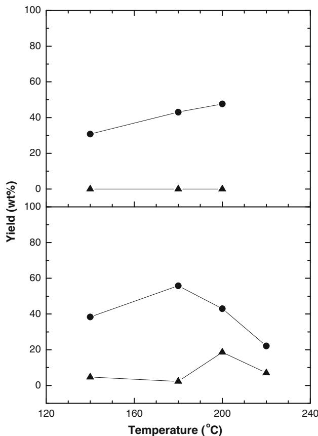
**Fig. 2** Yields of MG (closed circle) and DMDG (closed triangle) with temperature over ZSM-5(55) (top), and Y(30) (bottom). Catalyst/ $\text{CH}_2\text{O}$  = 0.2 and 0.4 respectively
