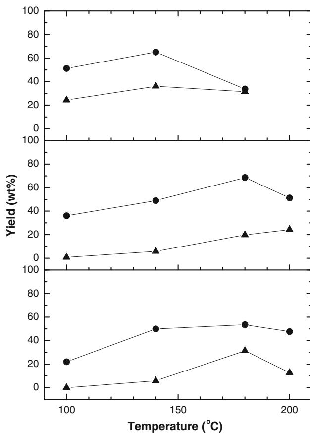
**Fig. 1** Yields of MG (closed circle) and DMDG (closed triangle) with temperature. over HPW (top), Amberlyst-15 (middle), and Amberlyst-70 (bottom). Catalyst/CH<sub>2</sub>O = 0.23, 0.4 and 0.67 respectively
