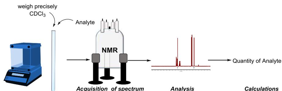
**Figure 1.** (A) NMR internal standard should be added to each sample. (B) No need for the addition of extra internal standard after the determination of residual  $\text{CHCl}_3$  concentration in  $\text{CDCl}_3$ .
