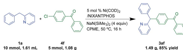
Scheme 5 Gram scale reaction via nickel-catalyzed DCCP reaction.
