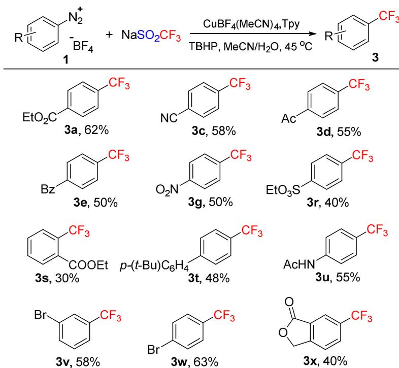
**Scheme 3.** Substrate scope of copper-mediated trifluoromethylation of arenediazonium tetrafluoroborates. Reaction conditions: **1** (0.2 mmol), NaSO<sub>2</sub>CF<sub>3</sub> (0.6 mmol), CuBF<sub>4</sub>(MeCN)<sub>4</sub> (0.4 mmol), Tpy (0.4 mmol), MeCN/H<sub>2</sub>O (2.0 mL/0.1 mL), 45 °C, under N<sub>2</sub>, overnight. Yields are those of the isolated products.
