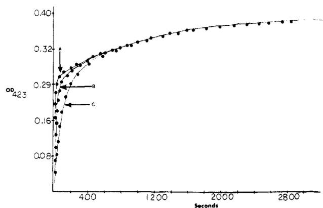
**Figure 1.** Absorbance (423 nm) vs. time (s) plots for the reduction of NMM by  $1 \times 10^{-5}$  M PPTH<sub>2T</sub> in 1.0 M pH 5.50 acetate buffer,  $\mu = 1.0$  KCl, at 30 °C under argon. [NMM] =  $1.67 \times 10^{-2}$  M (A),  $8.39 \times 10^{-3}$  M (B), and  $4.19 \times 10^{-3}$  M (C).
