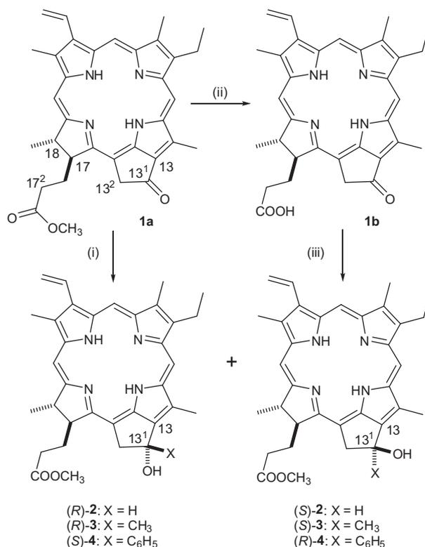
**Scheme 4.** Reaction of the 13-C=O in pyropheophorbides **1** to carbinols (*R/S*)-**2-4**. Reagents and conditions: (i) NaBH<sub>4</sub>/CH<sub>2</sub>Cl<sub>2</sub>-MeOH or *l*-selectride/THF, rt; (ii) H<sub>2</sub>SO<sub>4</sub>/H<sub>2</sub>O-THF; (iii) CH<sub>3</sub>Li/Et<sub>2</sub>O or C<sub>6</sub>H<sub>5</sub>Li/Bu<sub>2</sub>O, TMEDA/THF, -40 or -60 °C to rt and CH<sub>2</sub>N<sub>2</sub>/Et<sub>2</sub>O.
