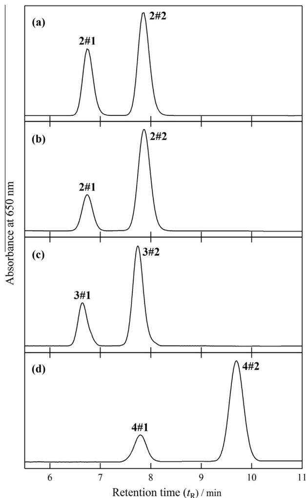
**Fig. 2.** RP-HPLC of (a) **2#1/2** (= **2(R)/(S)-2**, by NaBH<sub>4</sub>), (b) **2#1/2** (= **2(R)/(S)-2**, by *l*-selectride), (c) **3#1/2** (= **(R/S)-3**), and (d) **4#1/2** (= **(R/S)-4**). Conditions: Cosmosil 5C<sub>18</sub>-AR-II (4.6 mm  $\phi$   $\times$  150 mm), MeOH/H<sub>2</sub>O = 95:5 (v/v), and 1.0 mL/min.
