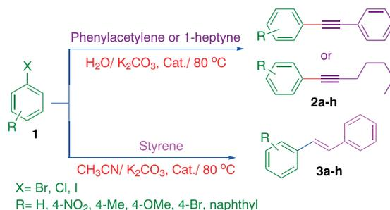
**Scheme 2.** Applicability of the novel Pd-based catalyst in C–C coupling reactions.
