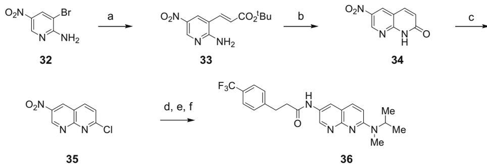
**Scheme 3.** Reagents and conditions: (a) *tert*-butyl acrylate, Pd(OAc)<sub>2</sub>, (*o*-tol)<sub>3</sub>P, Et<sub>3</sub>N/DMF, 130 °C; (b) 5 N aq HCl, sealed tube, 130 °C; (c) POCl<sub>3</sub>, reflux; (d) *N*-methylisopropylamine, K<sub>2</sub>CO<sub>3</sub>, DMF, 80 °C; (e) H<sub>2</sub>, Pd-C, MeOH; (f) RCOCl, Et<sub>3</sub>N, CH<sub>2</sub>Cl<sub>2</sub>.
