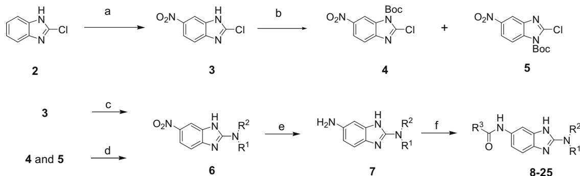
**Scheme 1.** Reagents and conditions: (a) 70% HNO<sub>3</sub>, H<sub>2</sub>SO<sub>4</sub>; (b) Boc<sub>2</sub>O, DMAP, THF; (c) R<sup>1</sup>R<sup>2</sup>NH (8–50 equiv), neat or in dioxane, sealed tube, 130 °C; (d) R<sup>1</sup>R<sup>2</sup>NH or HCl salt (2.2–3.3 equiv), DIEA, dioxane or DMSO, 80–100 °C; (e) H<sub>2</sub>, Pd(OH)<sub>2</sub>-C, MeOH; (f) R<sup>3</sup>COOH, HATU, DIEA, CH<sub>2</sub>Cl<sub>2</sub> or R<sup>3</sup>COCl, Et<sub>3</sub>N, CH<sub>2</sub>Cl<sub>2</sub>.
