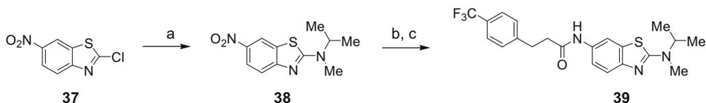
**Scheme 4.** Reagents and conditions: (a) *N*-methylisopropylamine (3 equiv), K<sub>2</sub>CO<sub>3</sub>, DMF, 80 °C; (b) H<sub>2</sub>, Pd-C, MeOH/THF; (c) RCOOH, 2-chloro-1,3-dimethylimidazolidinium chloride, pyridine, CHCl<sub>3</sub>.
