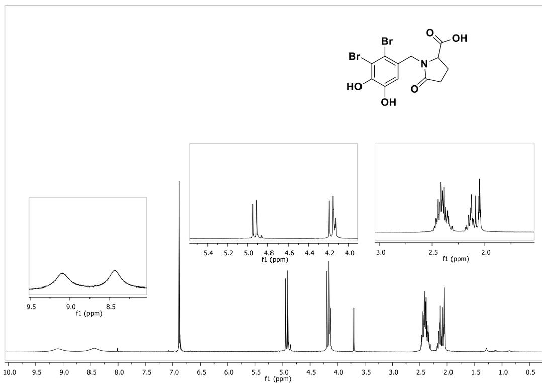
$^1\text{H}$  NMR spectrum of compound 3 (400 MHz, Acetone- $\text{d}_6$ )
