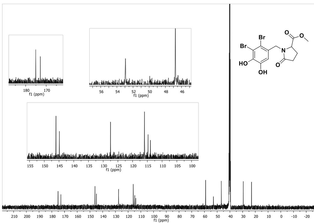
$^{13}\text{C}$  NMR spectrum of compound 4 (100 MHz, Acetone- $d_6$ )
