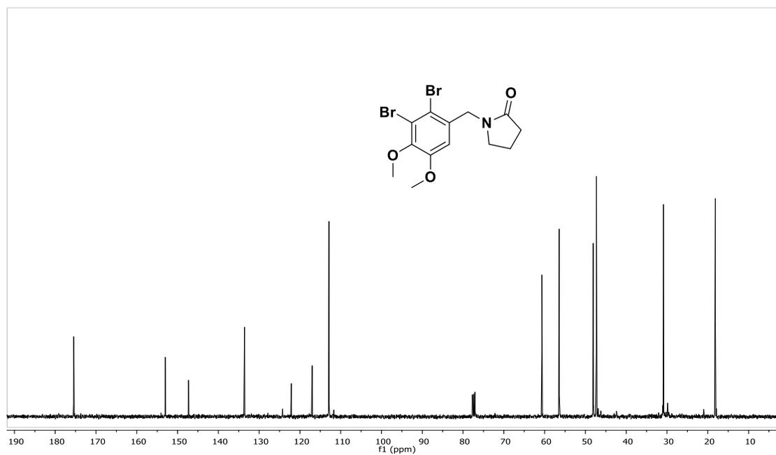
$^{13}\text{C}$ -NMR spectrum of compound 10 (100 MHz,  $\text{CDCl}_3$ )
