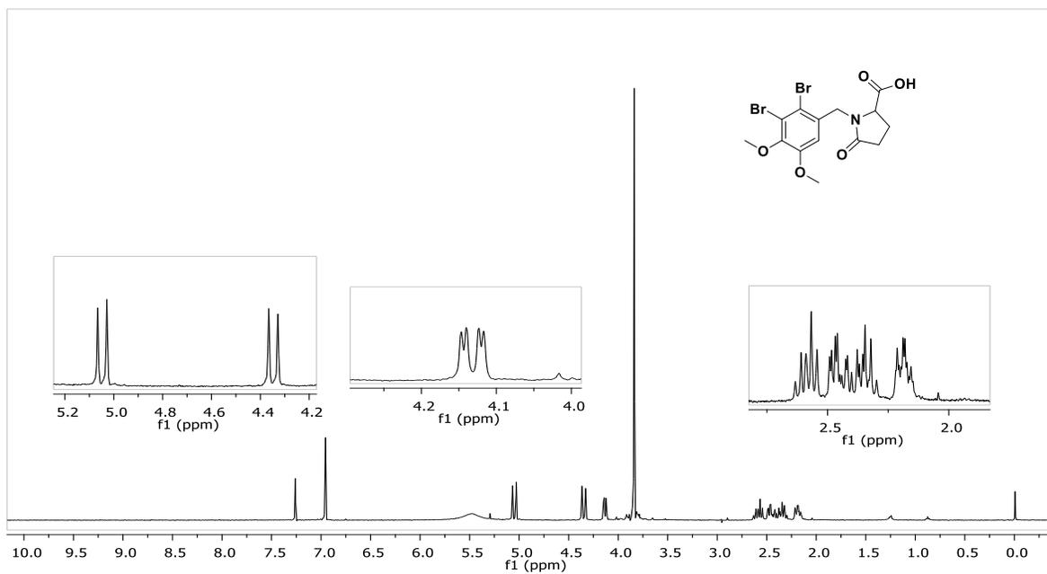
$^1\text{H}$  NMR spectrum of compound **8** (400 MHz,  $\text{CDCl}_3$ )
