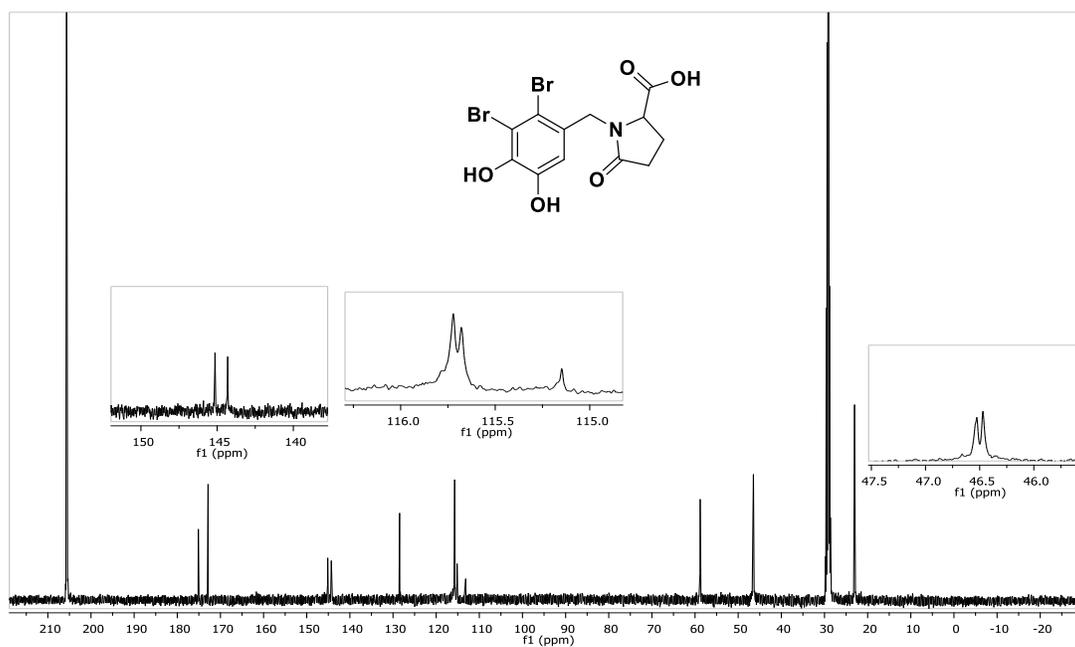
$^{13}\text{C}$  NMR spectrum of compound 3 (100 MHz, Acetone- $\text{d}_6$ )
