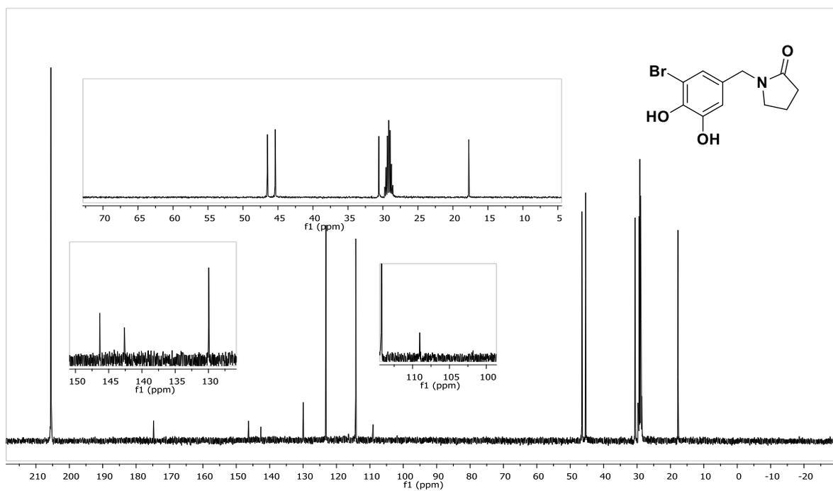
$^{13}\text{C}$  NMR spectrum of compound **16** (100 MHz, Acetone- $\text{d}_6$ )
