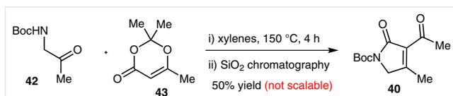
Scheme 12 Initial synthesis of unsaturated Boc-lactam 40
