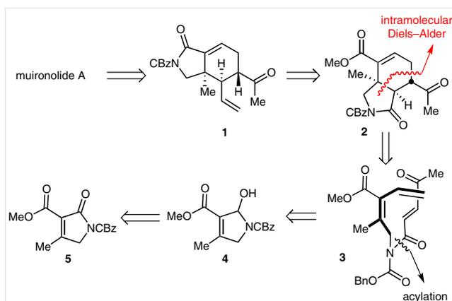
**Scheme 1** Intramolecular retrosynthetic analysis of muironolide A
