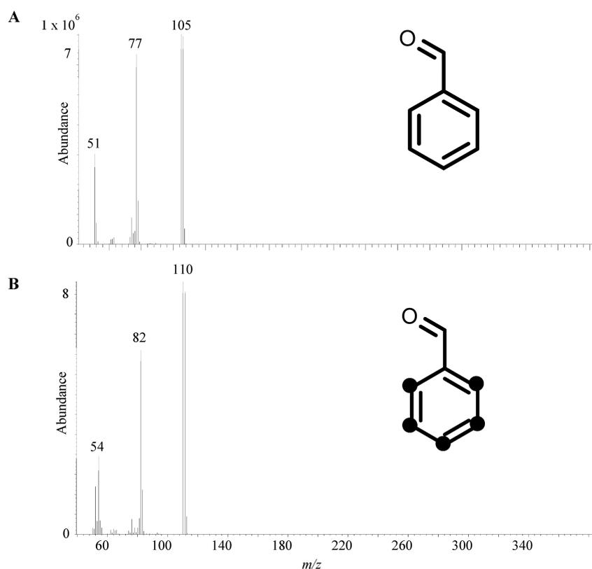
**Figure 1.** EI-MS spectra of (a) unlabeled and (b) labeled benzaldehyde produced when fermentations were incubated with ( $^2\text{H}_5$ )-benzyl alcohol.
