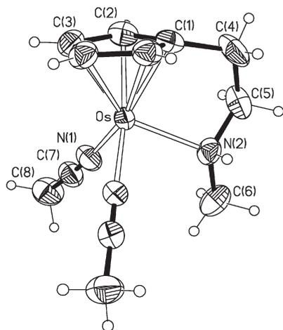
**Figure 2.** Molecular diagram of complex **4a**. Selected bond lengths (Å) and angles (deg): Os–C(1) 2.095(8); Os–C(2) 2.144(6); Os–C(3) 2.161(6); Os–N(1) 2.049(5); Os–N(2) 2.176(8); C(1)–Os–N(2) 82.3(3); N(1)–Os–N(2) 83.3(3).
