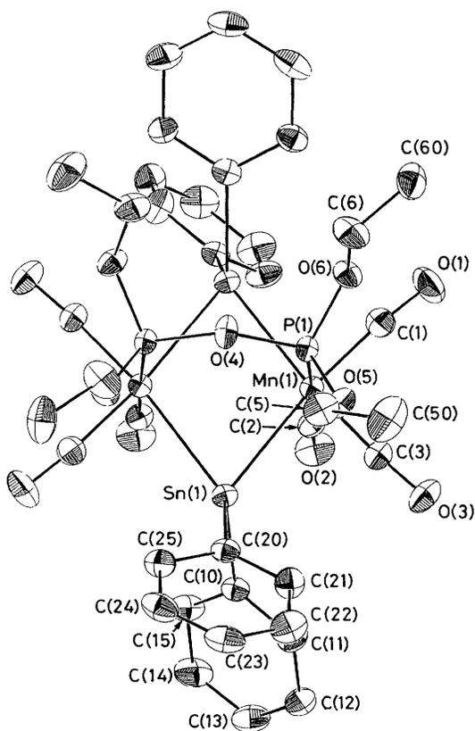
**Figure 2.** Molecular structure of  $[\text{Mn}_2(\mu\text{-SnPh}_2)_2(\text{CO})_6(\mu\text{-tedip})]$  (**5b**). Bond distances (Å): Mn(1)–Mn'(1) 3.1045(5), Mn(1)–Sn(1) 2.6053(5), Mn'(1)–Sn(1) 2.6178(6), Mn(1)–P(1) 2.2472(4). Bond angles (°): Mn(1)–Sn(1)–Mn'(1) 72.94(2), Sn(1)–Mn(1)–Sn(1) 106.93(2), C(10)–Sn(1)–C(20) 98.6(1), P(1)–Mn(1)–Sn(1) 91.49(3).
