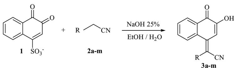
Scheme 1. Synthesis of 2-hydroxynaphthoquinomethanes in aqueous solvent.
