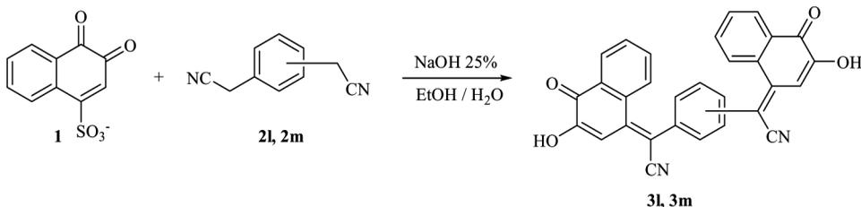
**Scheme 2.** Synthesis of bis-hydroxynaphthoquinones.
