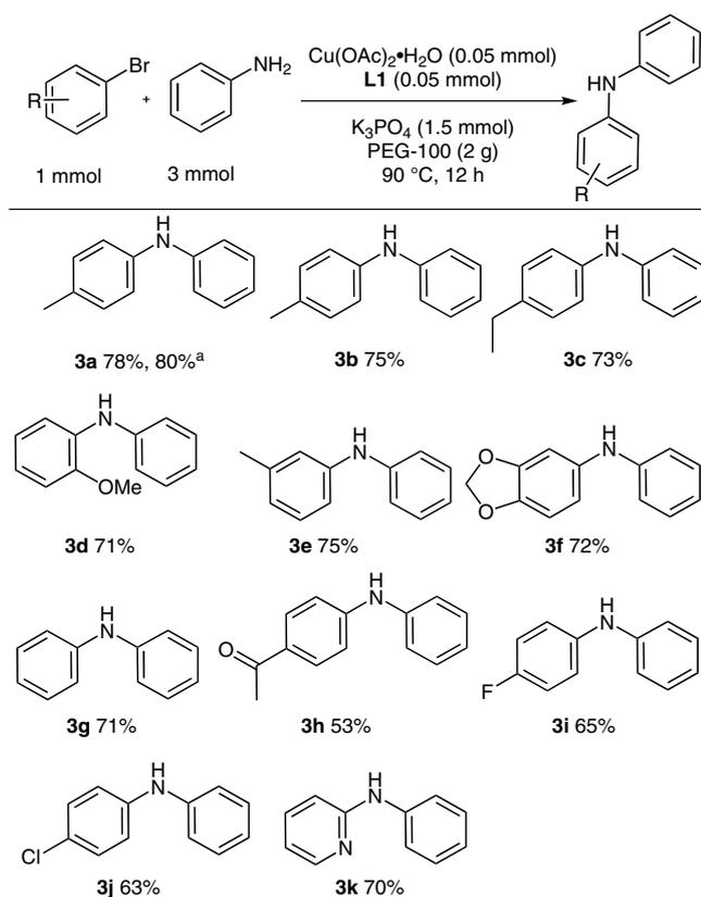
**Scheme 2** Products and isolated yields for amination of aryl bromides with aniline. <sup>a</sup> 4-Iodoanisole was used.
