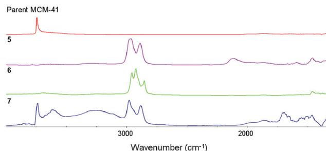
Fig. 5 IR spectra (DRIFT) of the parent material MCM-41, Ce[N(SiHMe<sub>2</sub>)<sub>2</sub>]<sub>4</sub>@MCM-41 (5), Ce[N(SiMe<sub>3</sub>)<sub>2</sub>]<sub>3</sub>Cl (6) and CeCp<sub>3</sub>Cl@MCM-41 (7) in the range 1300–4000 cm<sup>-1</sup>.
