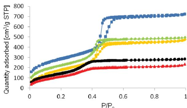
**Fig. 6** Nitrogen adsorption-desorption isotherms of MCM-41 parent material (blue squares), HN(SiHMe<sub>2</sub>)<sub>2</sub>@MCM-41 (green diamonds), Ce[N(SiHMe<sub>2</sub>)<sub>2</sub>]<sub>4</sub>@MCM-41 (5, black circles), Ce[N(SiMe<sub>3</sub>)<sub>2</sub>]<sub>3</sub>Cl@MCM-41 (6, red triangles), and Cp<sub>3</sub>CeCl@MCM-41 (7, orange circles).
