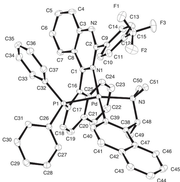
**Figure 2.** X-ray structure of (*S,R*)-**14** (H atoms and CDCl<sub>3</sub> solute have been removed for clarity). Selected distances (Å) and angles (°): Pd–P1 2.2608(5), Pd–N1 2.178(2), Pd–N3 2.140(2), Pd–C39 1.995(2), Pd···C10 3.048(2), P1–Pd–N1 84.0(1), P1–Pd–N3 157.3(1), N1–Pd–C39 173.6(1).
