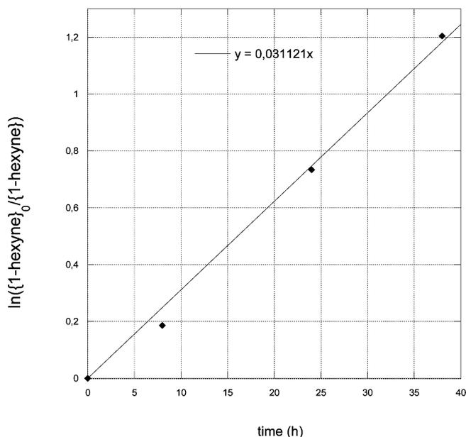
**Figure 2.** Plot of  $\ln([1\text{-hexyne}]_0/[1\text{-hexyne}])$  versus time (h) for the hydroamination reaction of 1-hexene by aniline catalyzed by the Ga species **2**. Conditions: [1-hexene]<sub>0</sub> = [aniline]<sub>0</sub> = 0.156 M, 5 mol % of Ga species **2**, C<sub>6</sub>D<sub>6</sub>, 100 °C.
