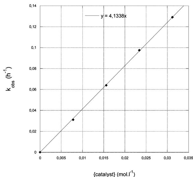
**Figure 3.** Plot of  $k_{\text{obs}}$  versus Ga species **2** concentration. Conditions: [1-hexyne]<sub>0</sub> = [aniline]<sub>0</sub> = 0.156 M, C<sub>6</sub>D<sub>6</sub>, 100 °C.
