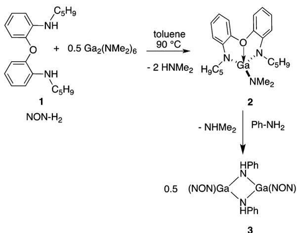
species  $\{\eta^3\text{-N,O,N-}((\text{C}_5\text{H}_9)\text{N-C}_6\text{H}_4)_2\text{O}\}\text{GaNMe}_2$  (**2**) may be directly prepared in a reasonable yield (51%) via an amine elimination route by reaction of the diamino-ether ligand **1** with 0.5 equiv of Ga<sub>2</sub>(NMe<sub>2</sub>)<sub>6</sub>. Compound **2** was isolated as an air- and moisture-sensitive colorless solid, and its molecular structure was confirmed by X-ray crystallography analysis.
