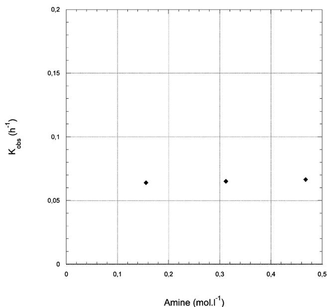
**Figure 4.** Plot of  $k_{\text{obs}}$  versus amine concentration for the hydroamination reaction of 1-hexyne by aniline catalyzed by the Ga species 2. Conditions:  $[1\text{-hexyne}]_0 = 0.156\text{ M}$ , 5 mol % of Ga species 2,  $\text{C}_6\text{D}_6$ ,  $100\text{ }^\circ\text{C}$ .
