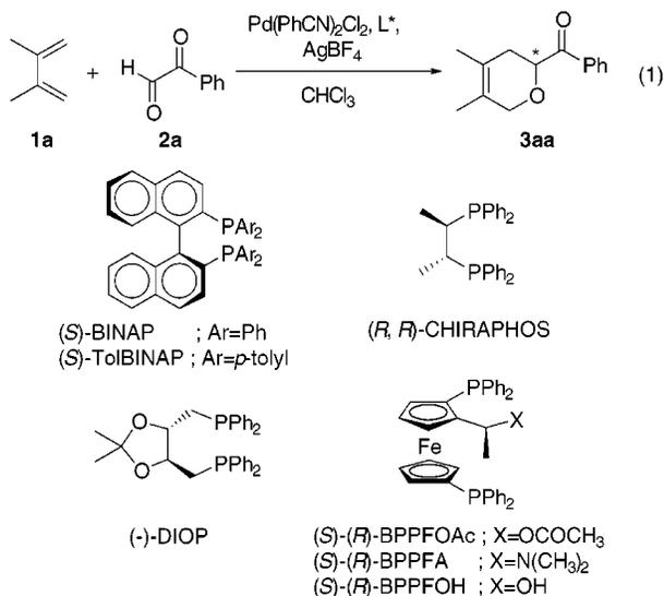
prepared in situ by mixing 2 mol % of Pd(PhCN)<sub>2</sub>Cl<sub>2</sub>, 1.0 equiv (for Pd) of the ligands, and 2.5 equiv (for Pd) of AgBF<sub>4</sub> prior to the reaction. The use of (*S*)-BINAP as the ligand of palladium gave product **3aa** in the highest yield, 69%, with the highest ee, 58% (entry 1). (*S*)-TolBINAP, which has *p*-tolyl groups attached to the phosphorus atoms instead of the phenyl groups found in (*S*)-BINAP,
