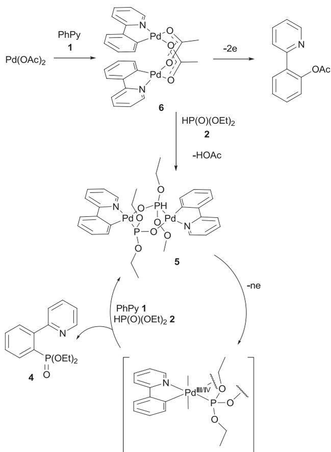
Scheme 3. Proposed catalytic cycle.
