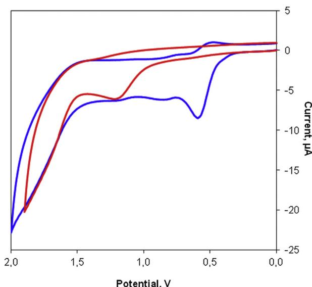
Fig. 2. Cyclic voltammograms of  $[(\text{PhPy})\text{Pd}(\mu\text{-OAc})_2]$  **2** (blue) and  $[(\text{PhPy})\text{Pd}(\text{EtO})_2\text{P}(\text{O})_2]$  **3** (red) vs.  $\text{Ag}/\text{AgNO}_3$  in  $\text{CH}_3\text{CN}$ . Scan rate 100 mV/s. (For interpretation of the references to color in this figure legend, the reader is referred to the web version of this article.)
