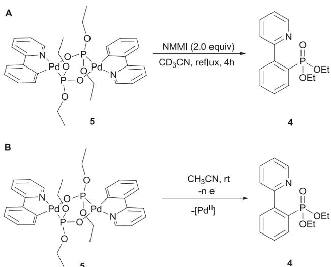
Scheme 2. Conversion of **5** into **4** in Murakami's reaction and under electrochemical oxidation.
