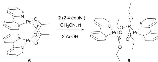
**Scheme 1.** Synthesis of [(PhPy)Pd(EtO)<sub>2</sub>P(O)]<sub>2</sub> palladacycle.
