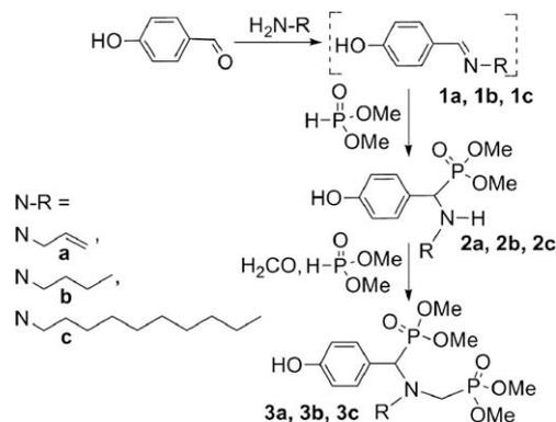
**Scheme 1.** Synthesis of phenol functionalized by azamonophosphonates (**2a-c**) and azadiphosphonates (**3a-c**).
