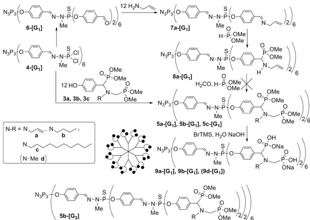
**Scheme 2.** Synthesis of dendrimers ended by azamonophosphonates (**8a-[G<sub>1</sub>]**), or non-symmetrical azadiphosphonates (**5a-[G<sub>1</sub>]**, **5a-[G<sub>2</sub>]**, **5b-[G<sub>1</sub>]**, **5c-[G<sub>1</sub>]**), or the sodium salt of non-symmetrical azadiphosphonic acids (**9a-[G<sub>1</sub>]**, **9b-[G<sub>1</sub>]**). Schematization of dendrimers **9-[G<sub>1</sub>]**. Compound **9d-[G<sub>1</sub>]** was previously reported.<sup>3a</sup>
