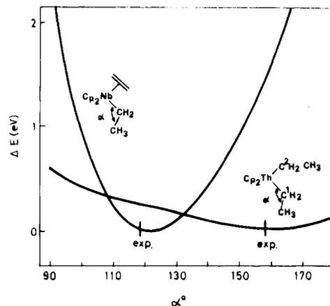
**Figure 1.** Potential energy curves of  $Cp_2Th(C_2H_5)_2$  and  $Cp_2Nb(H_2C=CH_2)(C_2H_5)$  as a function of M-C-C(ethyl) angle  $\alpha$ . The experimentally observed angle  $\alpha$  for  $Cp^*_2Th(CH_2CMe_3)_2$  or  $Cp_2Nb(H_2C=CH_2)(C_2H_5)$  is located by a mark "exp." in each corresponding curve.
