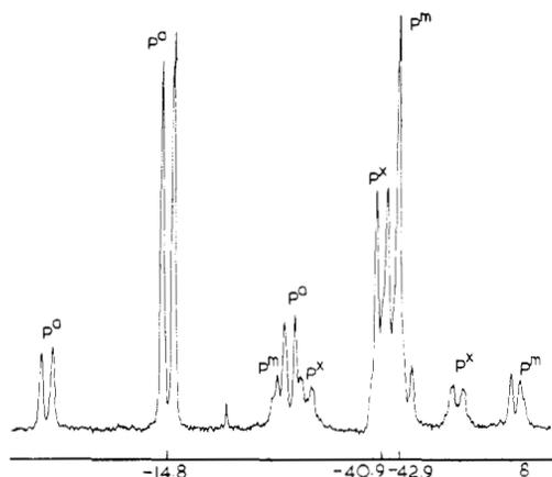
**Figure 2.**  $^{31}\text{P}\{^1\text{H}\}$  NMR spectrum (121.5 MHz) of complex **4a** at  $-90\text{ }^\circ\text{C}$ .
