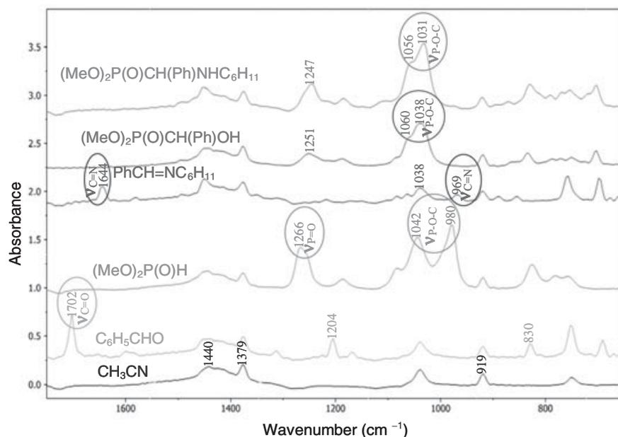
FIGURE 1 IR spectra of the reaction components measured in acetonitrile solution.
