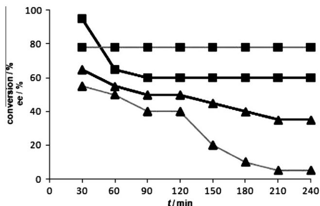
**Figure 1.** Conversion of the model aldol reaction as a function of time (black lines) in microreactors **R1** (■) and **R2** (▲). Enantioselectivity of the *anti*-aldol as a function of time (gray lines) in microreactors **R1** (■) and **R2** (▲).
