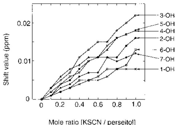
Fig. 4. Shifts in  $^1H$ -NMR Signals of Hydroxyl Protons of Perseitol (**1a**) (10.61 mg,  $1.67 \times 10^{-1} M$ ) by Adding KSCN
