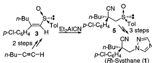
Highly enantiopure (*R*)-2-*p*-chlorophenyl-2-(1*H*-1,2,4-triazol-1-ylmethyl)hexanenitrile **1** (myclobutanil or systhane) was obtained in six synthetic steps from commercially available 1-hexyne (35% yield, 92% ee). The sulfinyl group controls the two key steps of the synthetic sequence, the highly stereoselective hydrocyanation of vinyl sulfoxides with Et<sub>2</sub>AlCN and the further introduction of the proper functionality into the molecule.
