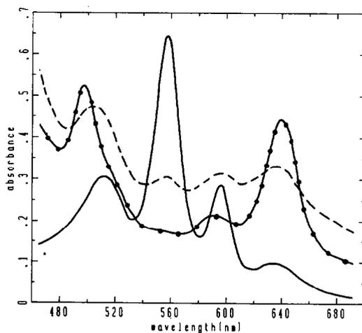
Fig. 4. The oxidation of ZnTPP by MCPBA catalyzed by  $1^+\text{Cl}^-$  in  $\text{CH}_3\text{OH}$ . —,  $3.6 \times 10^{-5}$  M ZnTPP and  $2 \times 10^{-6}$  M  $1^+\text{Cl}^-$  in  $\text{CH}_3\text{OH}$ ; ---, 20 sec after addition of  $10^{-3}$  M MCPBA;  $\odot \odot \odot$ , after 5 min.
