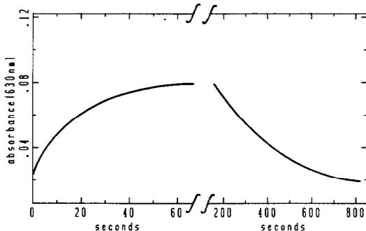
Fig. 9. The absorbance change at 630 nm vs time due to tri-*t*-butyl-phenoxy radical in  $\text{CH}_3\text{OH}$  upon addition of perlauric acid to a solution of TBPH,  $\text{I}^+\text{Cl}^-$  and 1,4-cyclohexadiene. The phenoxy radical is slowly quenched by the cyclohexadiene.  $[\text{I}^+\text{Cl}^-] = 1.2 \times 10^{-5}$  M; [TBPH] =  $5.5 \times 10^{-3}$  M; [perlauric acid] =  $1.4 \times 10^{-4}$  M; [cyclohexadiene] =  $10^{-1}$  M;  $T = 25^\circ$ .
