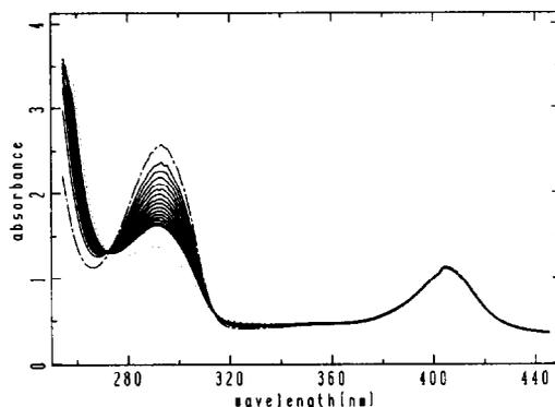
Fig. 6. Spectral changes occurring during  $1^+Cl^-$  catalyzed oxidation of hydroquinone by MCPBA. —, a solution of  $1 \times 10^{-3}$  M hydroquinone and  $8 \times 10^{-6}$  M  $1^+Cl^-$  in  $CH_3OH$ ; —, spectral changes from 3 to 45 sec at 3-sec intervals upon addition of  $8.8 \times 10^{-4}$  perlauric acid; ···, final spectrum after 120 sec.
