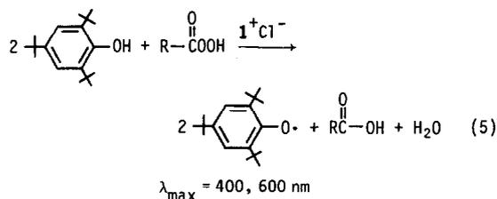
The stoichiometry of the reaction was found to be two moles of phenoxyl radical per mole of peracid as indicated by eqn (5) and the rate was first order in peracid, first order in chelated protohemin chloride, and zero order in phenol. Since this means the rate of intermediate formation is rate-limiting, we studied the structural and solvent effects on the formation reaction (eqn 6), in which  $\text{Hm}^+=\text{O}$  represents a species which is
