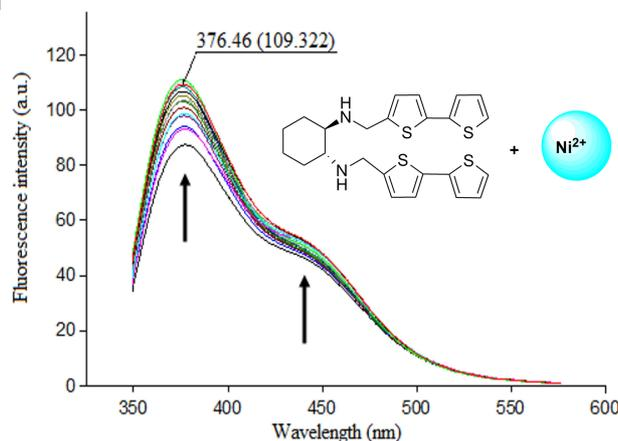
**Fig. 4.** Emission spectra of complex **3e** and  $\text{Ni}^{2+}$  (at 1:2 molar ratio in ethanol-water within 5 min).
