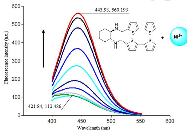
**Fig. 6.** The increase of fluorescence intensity in emission spectra of **3e** with  $\text{Ni}^{2+}$  in methanol (at molar ratio ligand / ion 2:1 within 10 min)
