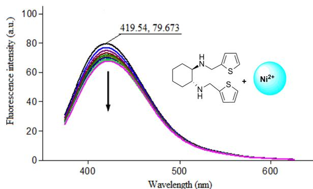
**Fig. 5.** The hypochromic effect in emission spectra of **3a** with  $\text{Ni}^{2+}$  in methanol (at molar ratio ligand / ion 2:1 within 1 h)
