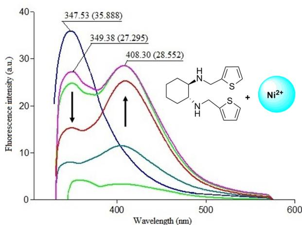
**Fig. 3.** Fluorescence emission spectra of complex **3a** and Ni<sup>2+</sup> (at 1:1 molar ratio, ethanol-water at 1:1 v/v within 5 min). The dark blue graph represents an initial emission spectrum of **3a**
