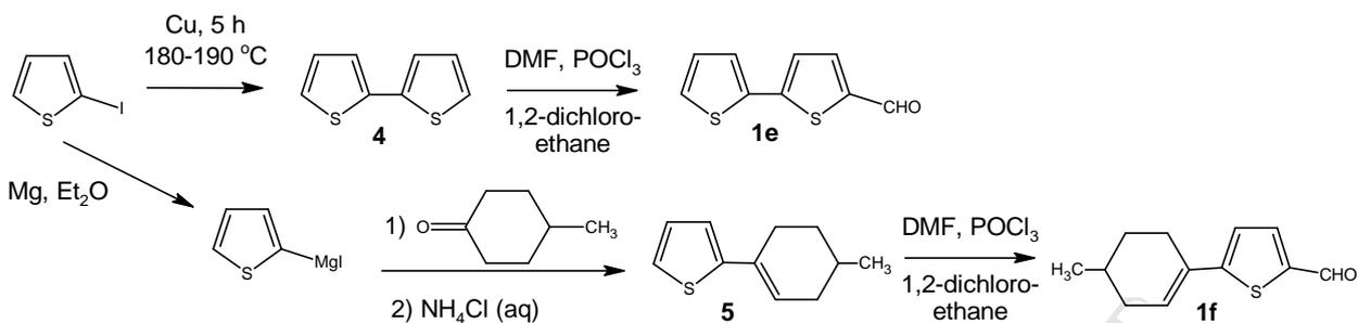
2,2'-Bithiophene (**4**) was prepared by improved Ulmann method<sup>1</sup>: a mixture of 2-iodothiophene (82 g, 0.39 mole) and copper (50 g, 0.78 mole) was refluxed (180 - 190°C) with stirring for 3 hours. The reaction mixture was extracted with 1,2-dichloroethane (3×200 ml) and copper iodide was removed by filtration. The solvent was removed with a rotary evaporator, the fractional distillation of the residue gave the *title compound* **4** (22.7 g, 70%); bp 102-108 °C/4 Torr)<sup>1</sup>.
