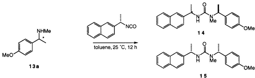
In several cases the enantiomer excess of the amine was measured by reaction with (*S*)-β-naphthylethyl isocyanate overnight to give the urea diastereomers **14** and **15** as a clear, colourless oil in 52-90% yield. In the <sup>1</sup>H NMR at 300MHz, the NCH<sub>3</sub>, OCH<sub>3</sub> (for the 4-OMe series) and ArCHCH<sub>3</sub> protons were distinct. For the amination of 4-methoxyphenylboronic ester **3a** using MeNHOSiMe<sub>3</sub> **5** and BuLi, the enantiomeric excess of the
