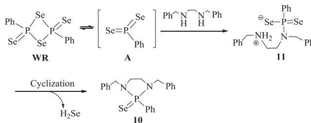
Scheme 5. A possible mechanism for the formation of compounds **10** and **11**.
