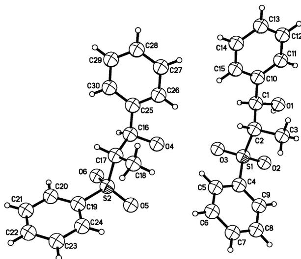
**Fig. 1** X-Ray crystal structure of the major diastereomer of **2a**.
